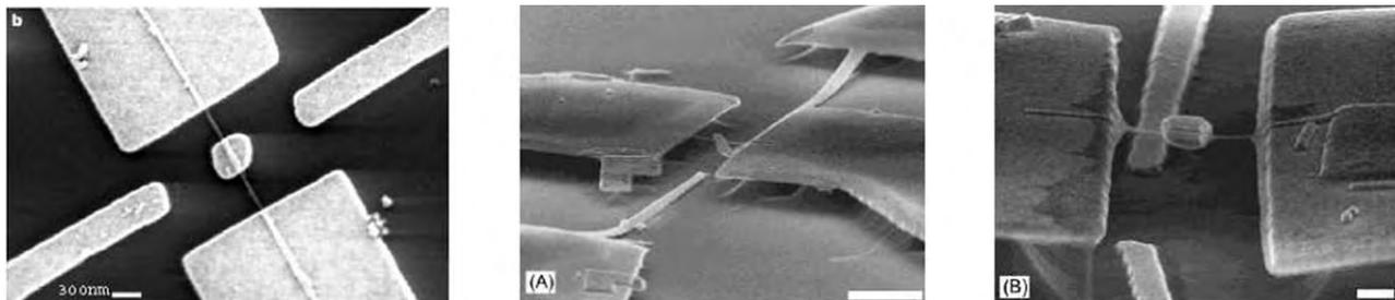
Figure 1. Nanoscale rotational actuators based on nanotubes built by: (a) Fennimore<sup>3</sup>, *et al.* (b) & (c) Bourlon<sup>8</sup>, *et al.*
