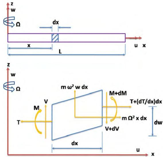
Figure 2. Forces acting on an incremental length  $dx$  of the rotating beam.
