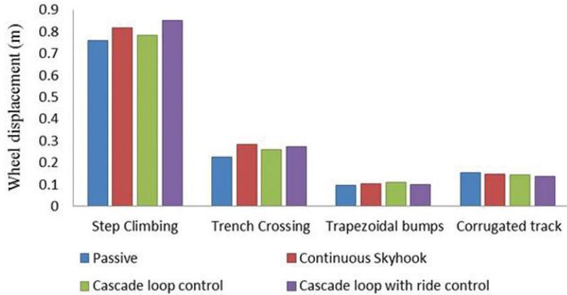
Figure 10. Comparison of actual wheel displacement (m) under various road inputs.
