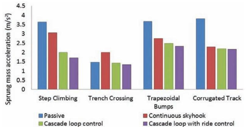
Figure 9. Comparison of RMS sprung mass acceleration ( $m/s^2$ ) under various road inputs.
