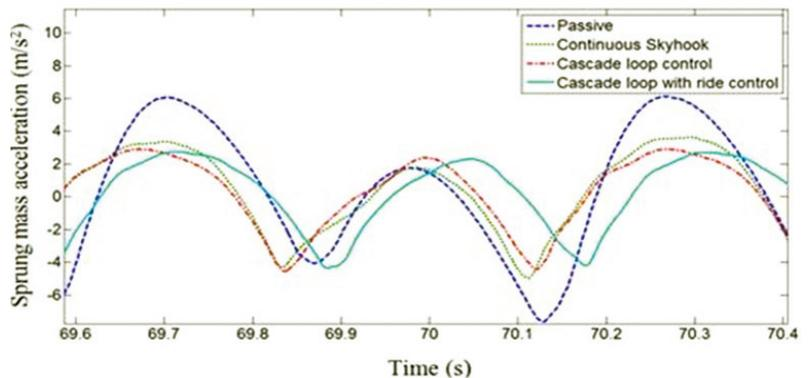
Figure 8. Comparison of the sprung mass acceleration without and with implementation of various control strategies during crossing corrugated track.
