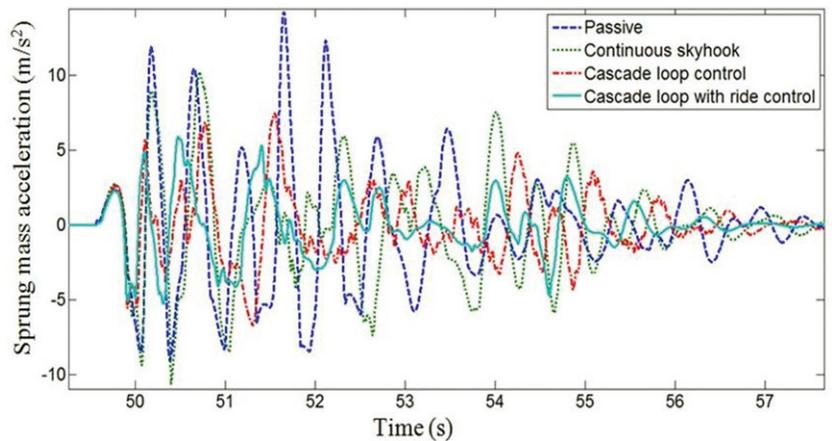
**Figure 5. Comparison of the sprung mass acceleration without and with implementation of various control strategies during step climbing.**
