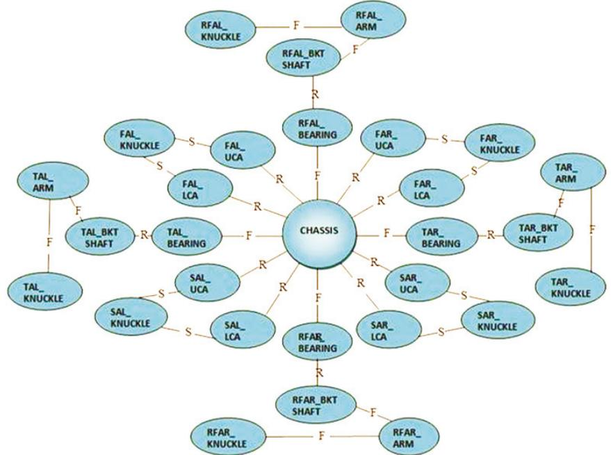
Figure 3. Topology map for suspension system.
