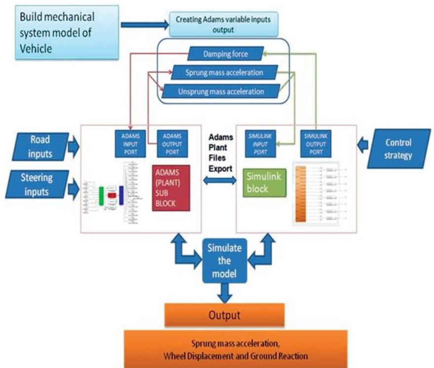
Figure 4. Co-simulation flow chart.
