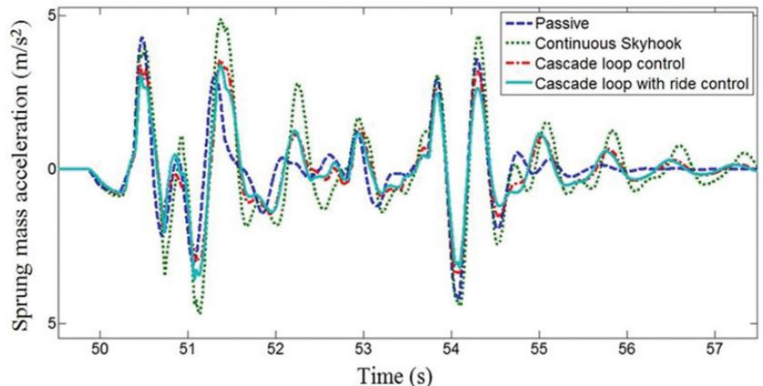
**Figure 6. Comparison of the sprung mass acceleration without and with implementation of various control strategies during trench crossing.**
