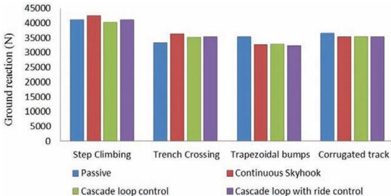
Figure 11. Comparison of RMS ground reaction (N) under various road inputs.
