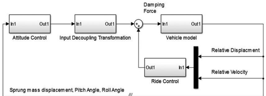
Figure 2. Control structure for cascade loop with ride control<sup>16</sup>.
