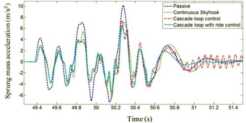
Figure 7. Comparison of the sprung mass acceleration without and with implementation of various control strategies during crossing trapezoidal bumps.
