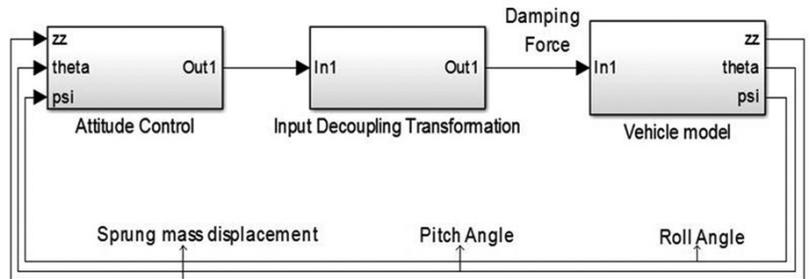
Figure 1. Control structure for cascade loop control<sup>16</sup>.
