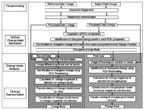
Figure 5. Block diagram depicting the improved CVA technique using enhanced PCA and inverse triangular function-based thresholding.
