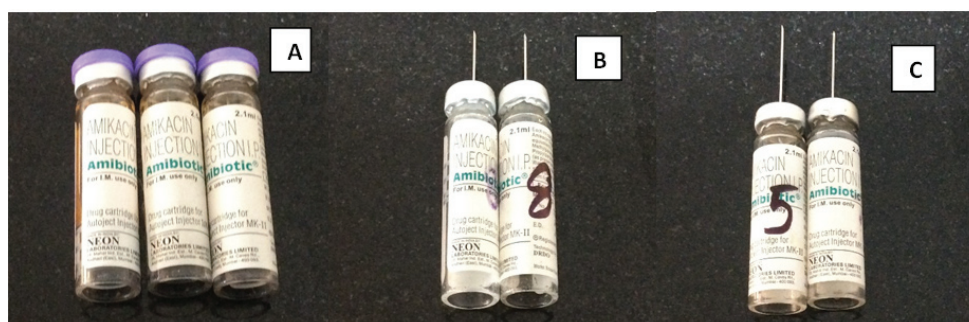
Figure 1. Amikacin drug cartridges for reusable autoinjector, (a) fresh cartridges, (b) partially ejected drug cartridges, and (c) fully ejected drug cartridges.
