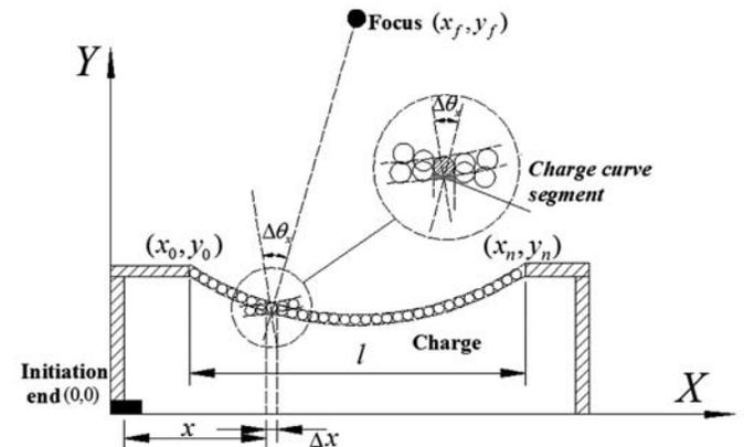
Figure 6. Design drawing of focusing warhead.
