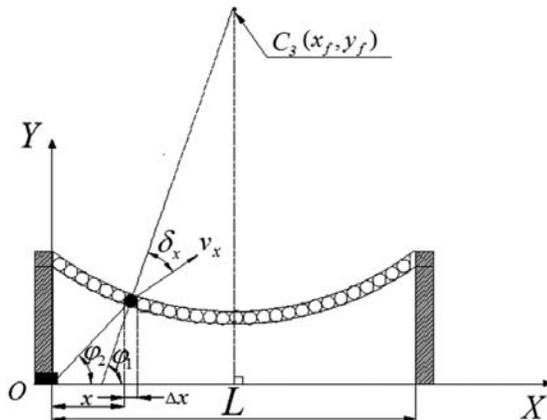
Figure 5. Elementary charge structure of focused fragmentation warhead.
