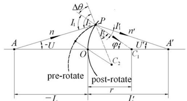
**Figure 4. Geometrical representation of refraction after spherical face was rotated by  $\Delta\theta$ .**
