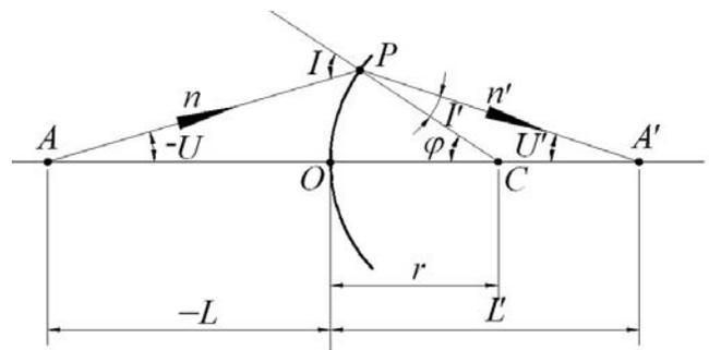
**Figure 3. Geometrical representation of refraction of a simple spherical surface.**
