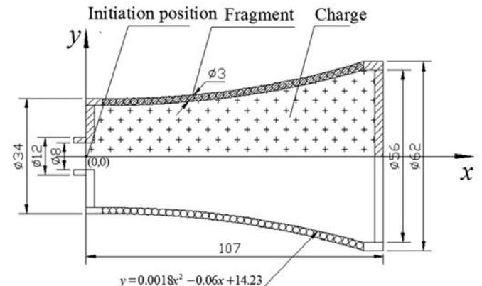
Figure 7. W-A scheme of focused fragmentation warhead.
