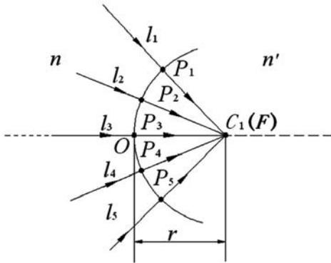
**Figure 1. Refraction at a simple spherical surface.**
