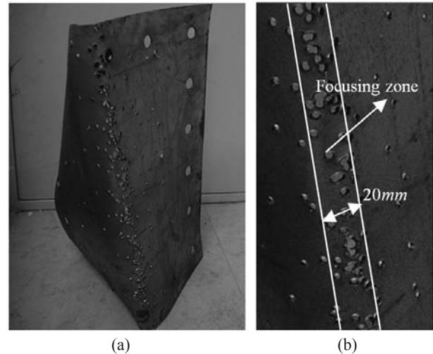
Figure 11. Distribution of fragments for W-A scheme: (a) Full view of target; (b) Detail of target.
