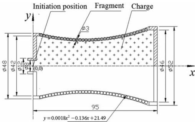
Figure 8. W-B scheme of focused fragmentation warhead.
