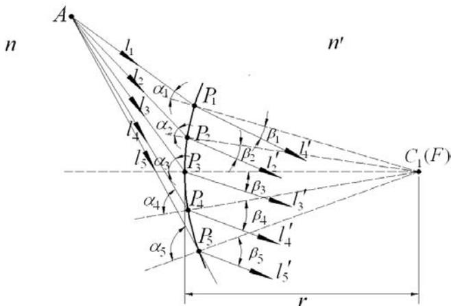
**Figure 2. Refraction of multiple lights at a simple spherical surface.**
