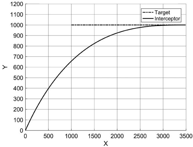
Figure 2. Intercept trajectory where the missile employs OPG for the non-maneuvering target case in the receding target scenario.
