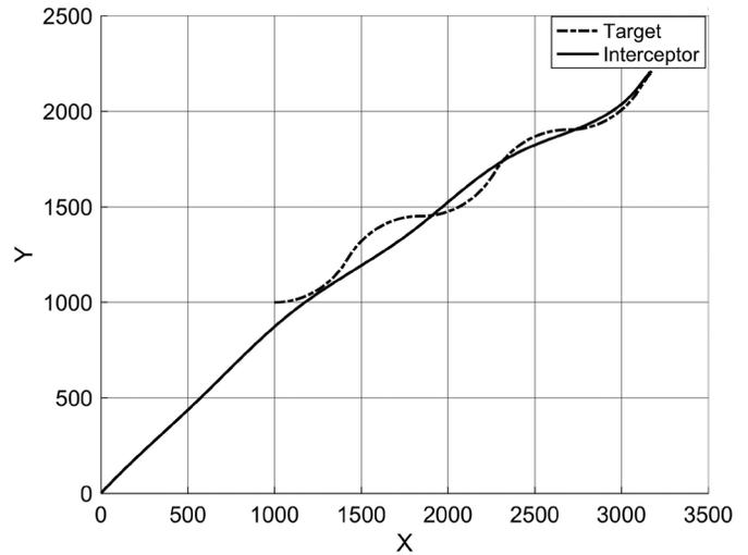
Figure 4. Intercept trajectory where the missile employs OPG for the switching coordinated turn case in the receding target scenario.
