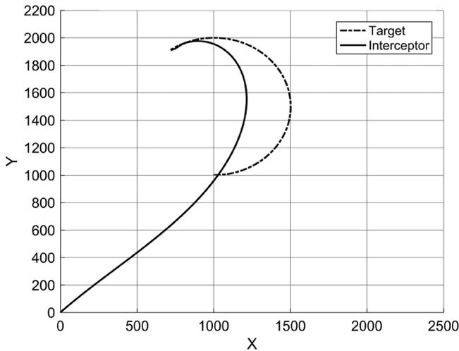
Figure 3. Intercept trajectory where the missile employs OPG for the coordinated turn case in the receding target scenario.
