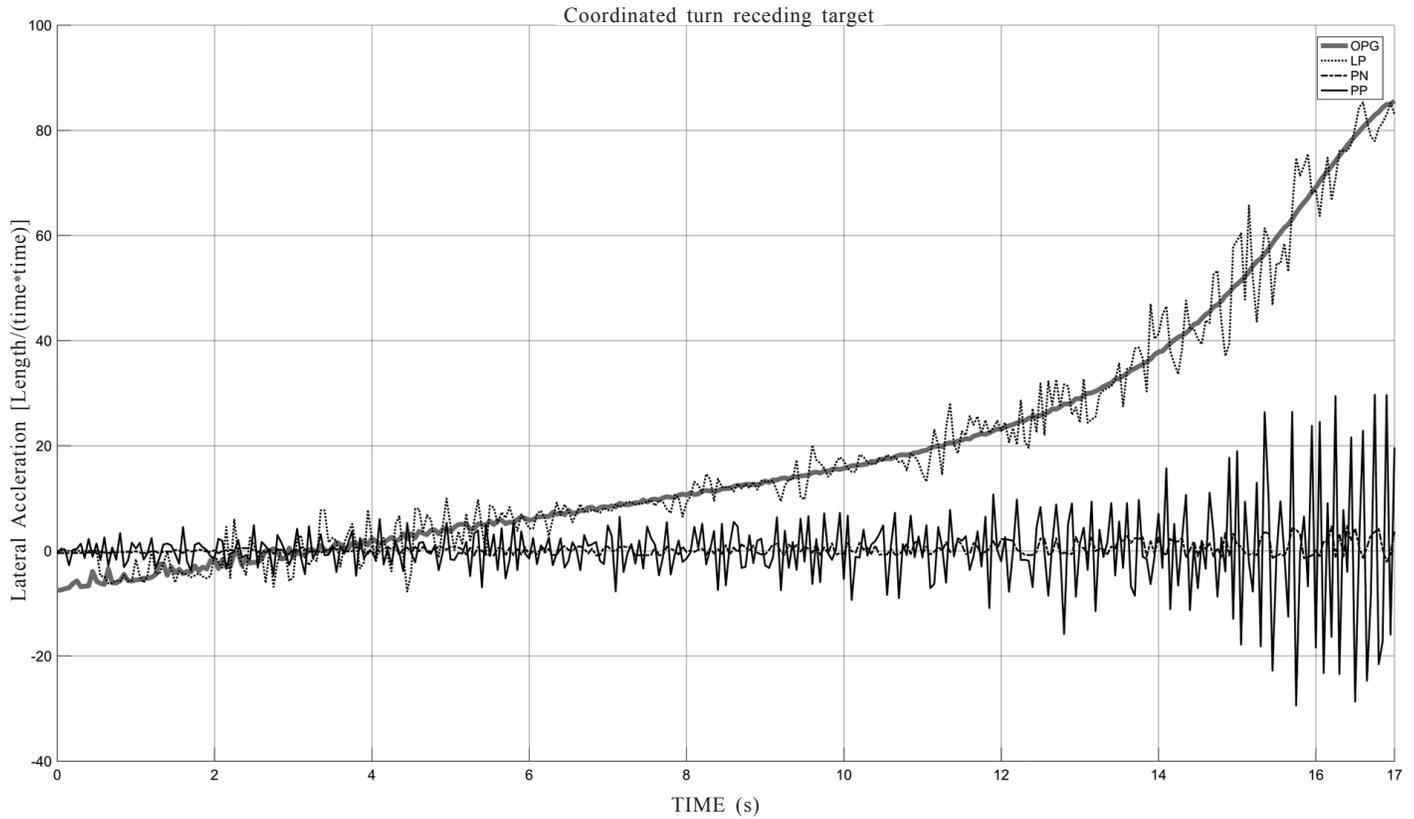
Figure 5. Interceptor lateral acceleration time histories of the considered guidance laws for the coordinated turn case in the receding target scenario.
