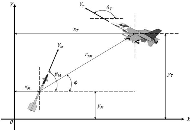
Figure 1. The missile-target engagement geometry.
