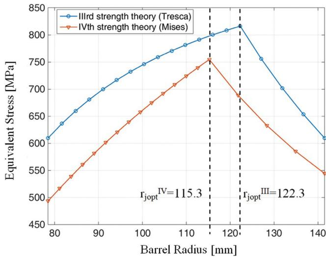
Figure 2. Comparison of equivalent stress based on III<sup>rd</sup> (Tresca) and IV<sup>th</sup> strength theories (Mises).
