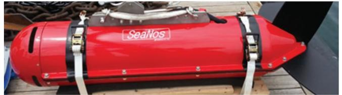
**Figure 3. Underwater acoustic signal maker, SeaNos, manufactured by KIOST.**
