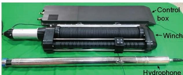
**Figure 2. Control box and winch for the 300-m fiber-optic cable.**
