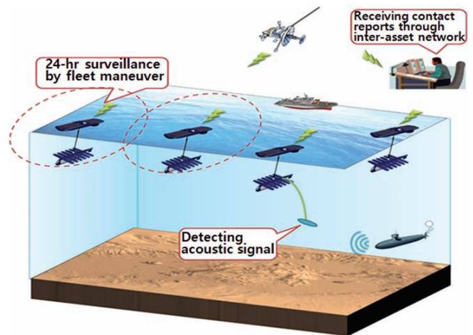
Figure 6. Schematic of an underwater surveillance network made up of multiple wave-powered unmanned surface vehicles.
