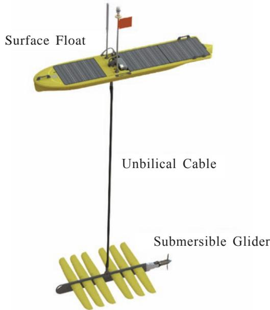
**Figure 1. Wave-powered glider (modified from liquid robotics Inc.).**
