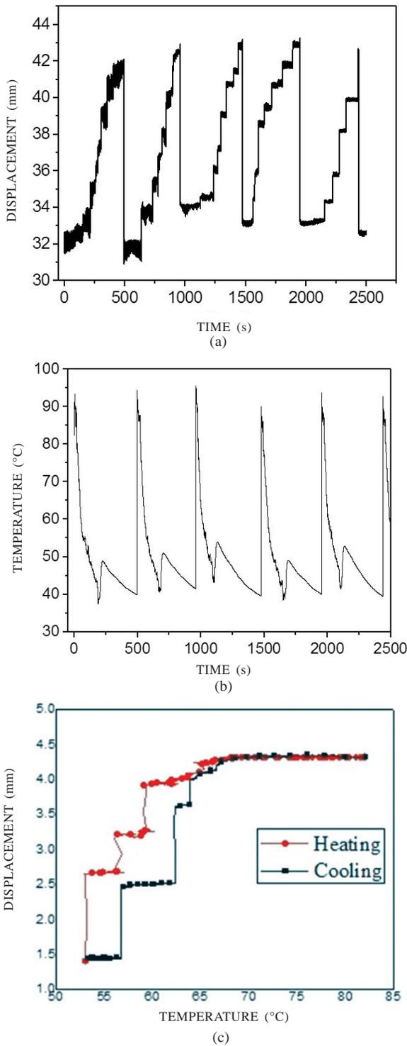
Figure 4. (a) Displacement vs time for 4.5 N load, (b) Temperature vs time for 4.5 N load, and (c) Displacement vs temperature for 4.5 N load.
