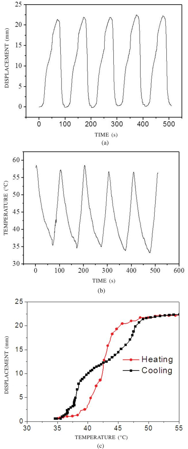
Figure 3. (a) Displacement versus time for 4.5 N load, (b) Temperature versus time for 4.5 N load, and (c) Displacement versus temperature for 4.5 N load.
