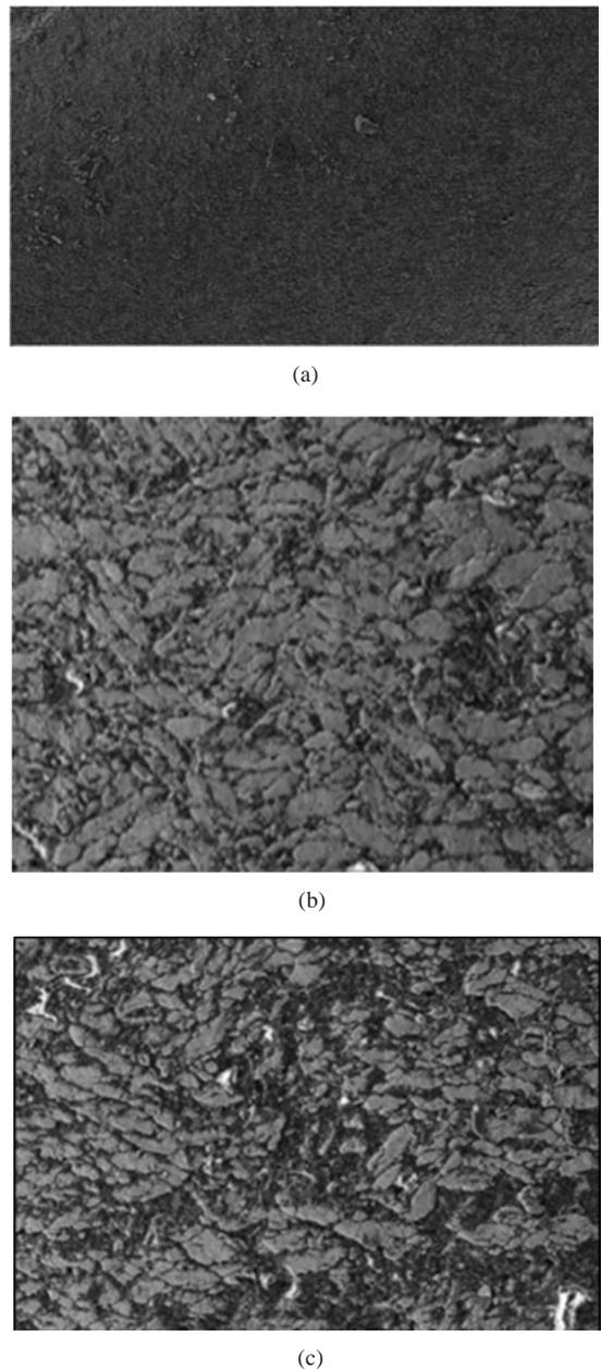
Figure 5. (a) SEM images for Non-Treated Ni-Ti, (b) SEM images for electrically actuated Ni-Ti, and (c) SEM images for hot water actuated Ni-Ti.
