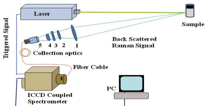
Figure 1. Schematic diagram of time gated Raman technique.
