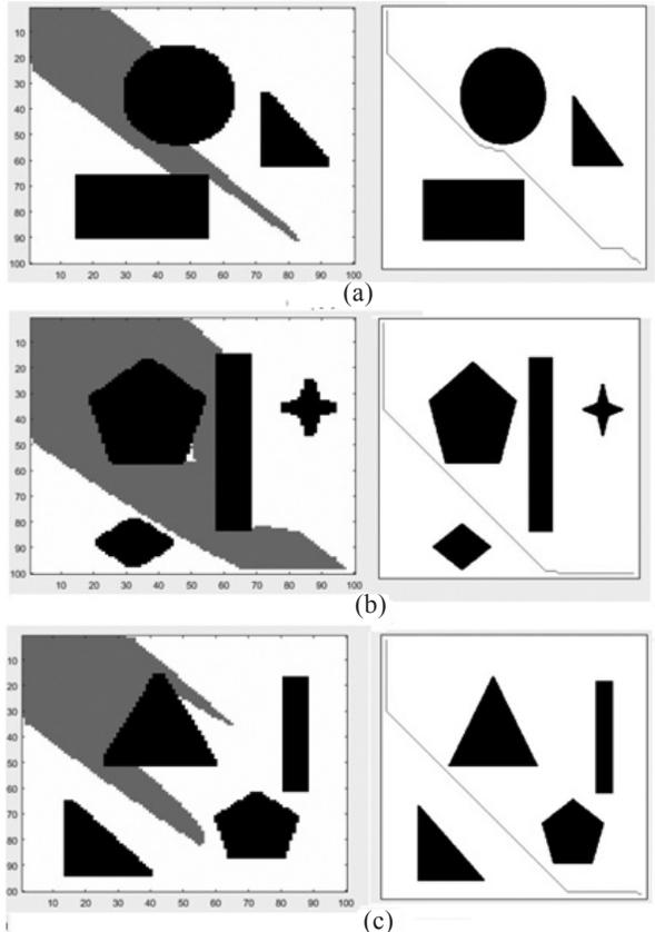
Figure 5. Snapshots of A\* star algorithm: (a) Map 1 in sequence 1, (b) Map 2 in sequence 1; (c) Map 1 in sequence 2.
