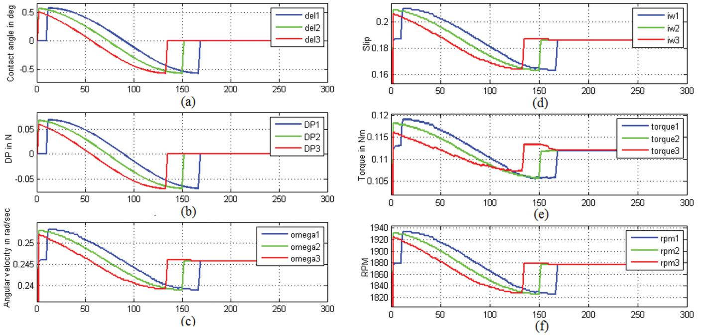
Figure 7. Estimation of angle, pull force, angular velocity, slip, torque and RPM.
