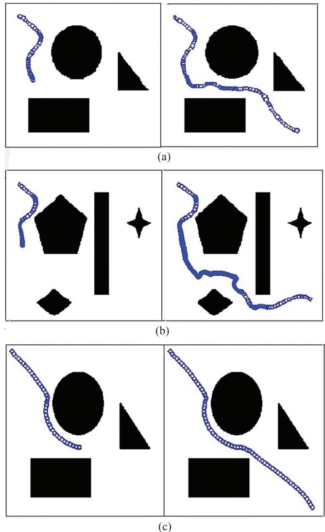
**Figure 6. Snapshots of: (a) Map 1 in potential field algorithm, (b) Following the searched path in potential field algorithm, and (c) Map 1 in fuzzy logic algorithm.**
