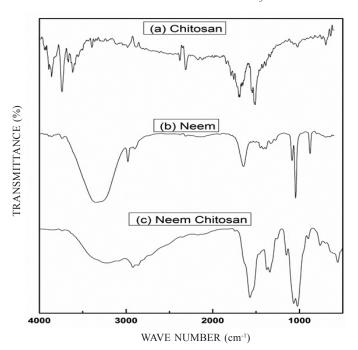
Figure 3. FT-IR spectrum of the hybrid system.
