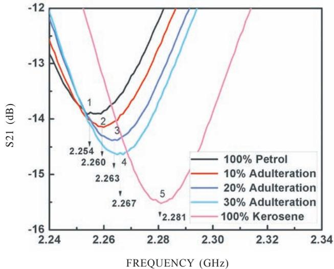
Figure 2. Shows the variation in S21 response for various adulterated concentrations of kerosene in petrol.
