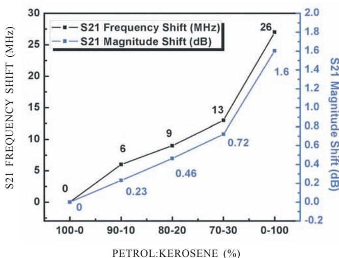
Figure 3. Shows the combined picture of the actual frequency and magnitude shifts wrt compositions of adulterated fuels.
