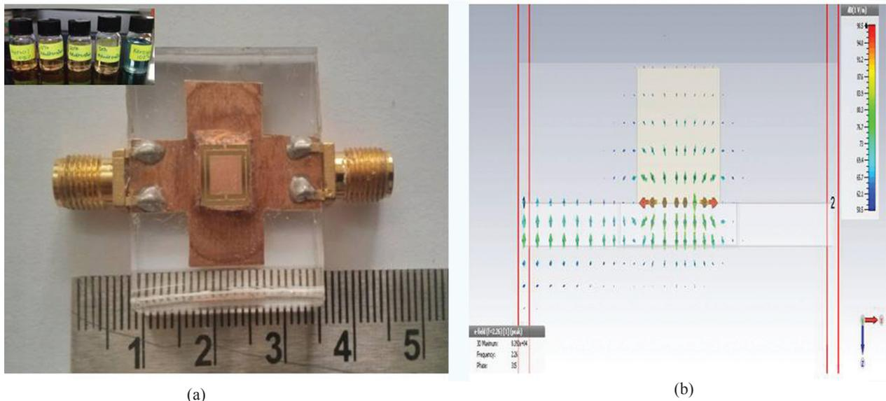
**Figure 1. (a) shows the CSRR device with the PDMS cavity along with photograph of fuel samples (inset) (b) Simulation of E-fields of CSRR cavity sensor.**
