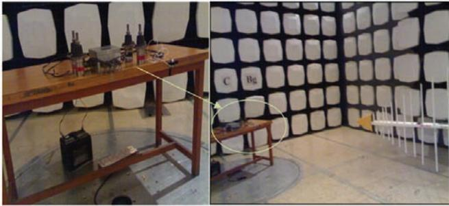
Figure 11. Experimental Setup for Electromagnetic radiation disturbance measurement in the microwave chamber.
