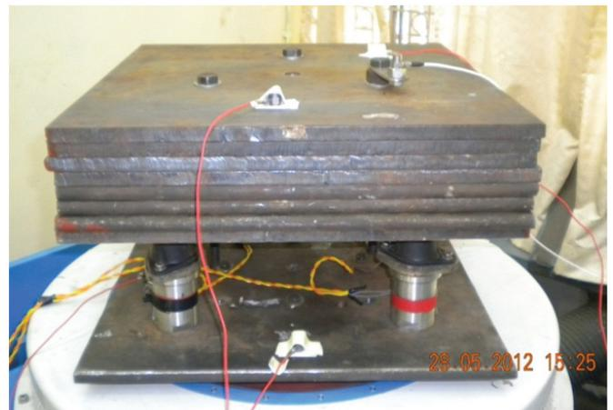
Figure 6. Experimental Set-up for carrying out vibration transmissibility tests.
