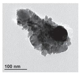
Figure 2. TEM of Nano-crystalline powder mechanically activated for 10 h (MA-10).
