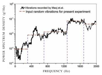
Figure 6. Random vibrations of aerospace vehicles along Z-axis<sup>28</sup>.
