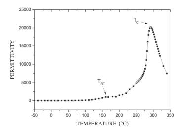
Figure 4. Temperature dependence of permittivity and phase transition behaviour.
