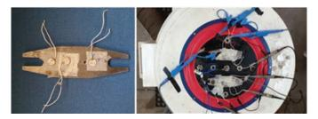
Figure 5. Fixture with components and vibration bench.
