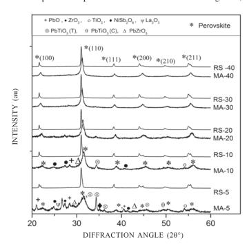
Figure 1. XRD pattern for mechanically activated (MA) Nanocrystalline powder samples and reactively sintered samples (RS).
