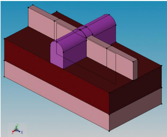
Figure 4. 3D view of the proposed triple gate device.
