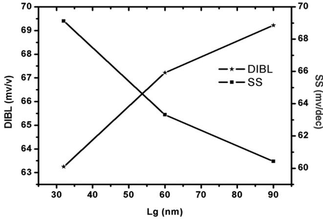
Figure 6. Gate length vs DIBL and sub-threshold slope.
