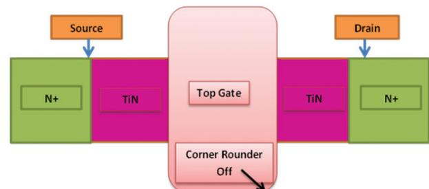
Figure 1. Top view of the proposed triple gate device.
