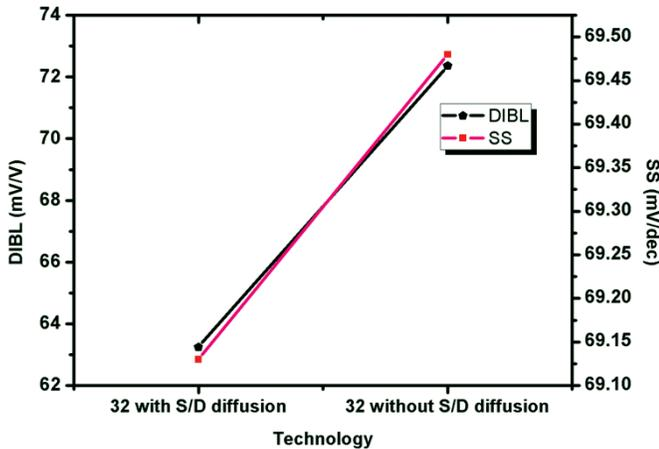
Figure 7. Comparison of DIBL and SS w.r.t. metal diffusion in source/drain.
