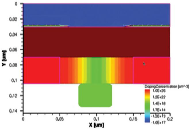
Figure 2. Corner rounded gate structure.
