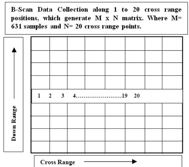
**Figure 3. B-scan data collection as stacking of A-scan.**
