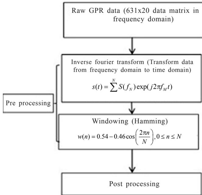
Figure 4. Flow diagram of GPR signal processing<sup>24</sup>.
