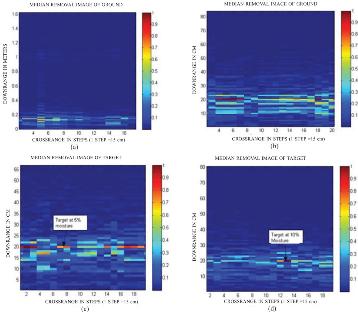
Figure 8. Median removal method: (a) without target (5% moisture) (b) without target (10 % moisture) (c) with target at 35 cm (5% moisture), and (d) with target at 35 cm (10% moisture).
