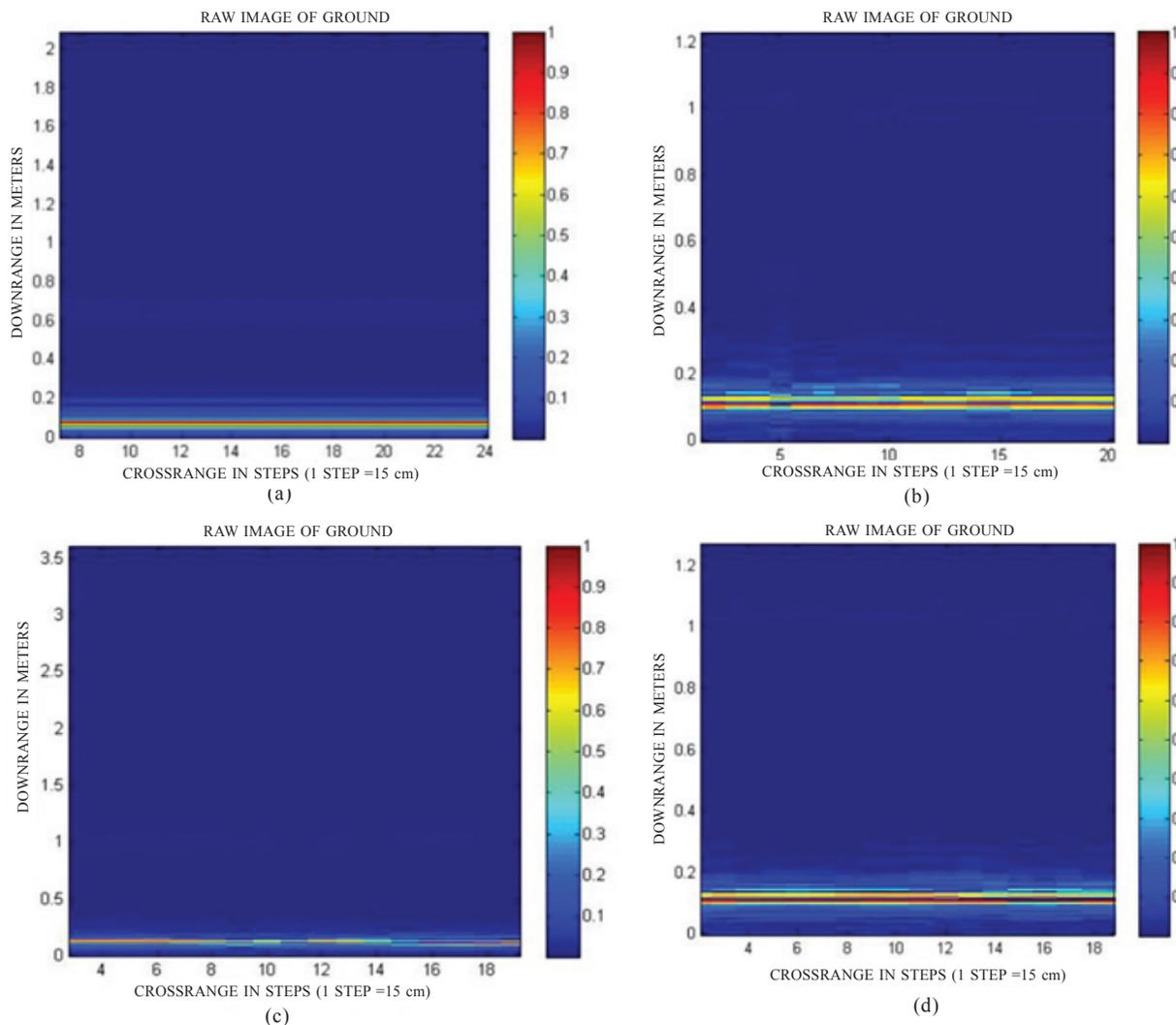
Figure 5. Raw images without and with target : (a) raw image without target (5 % moisture) (b) raw image without target (10 % moisture), (c) raw image with target (5 % moisture), and (d) raw image with target (10 % moisture).
