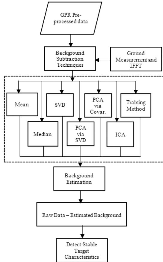
Figure 6. GPR data background subtraction flow.
