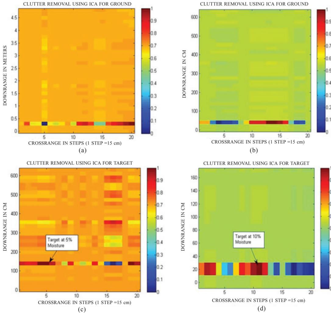
**Figure 12. ICA method: (a) without target (5% moisture), (b) without target (10 % moisture), (c) with target at 35 cm (5% moisture), and (d) with target at 35 cm (10% moisture).**
