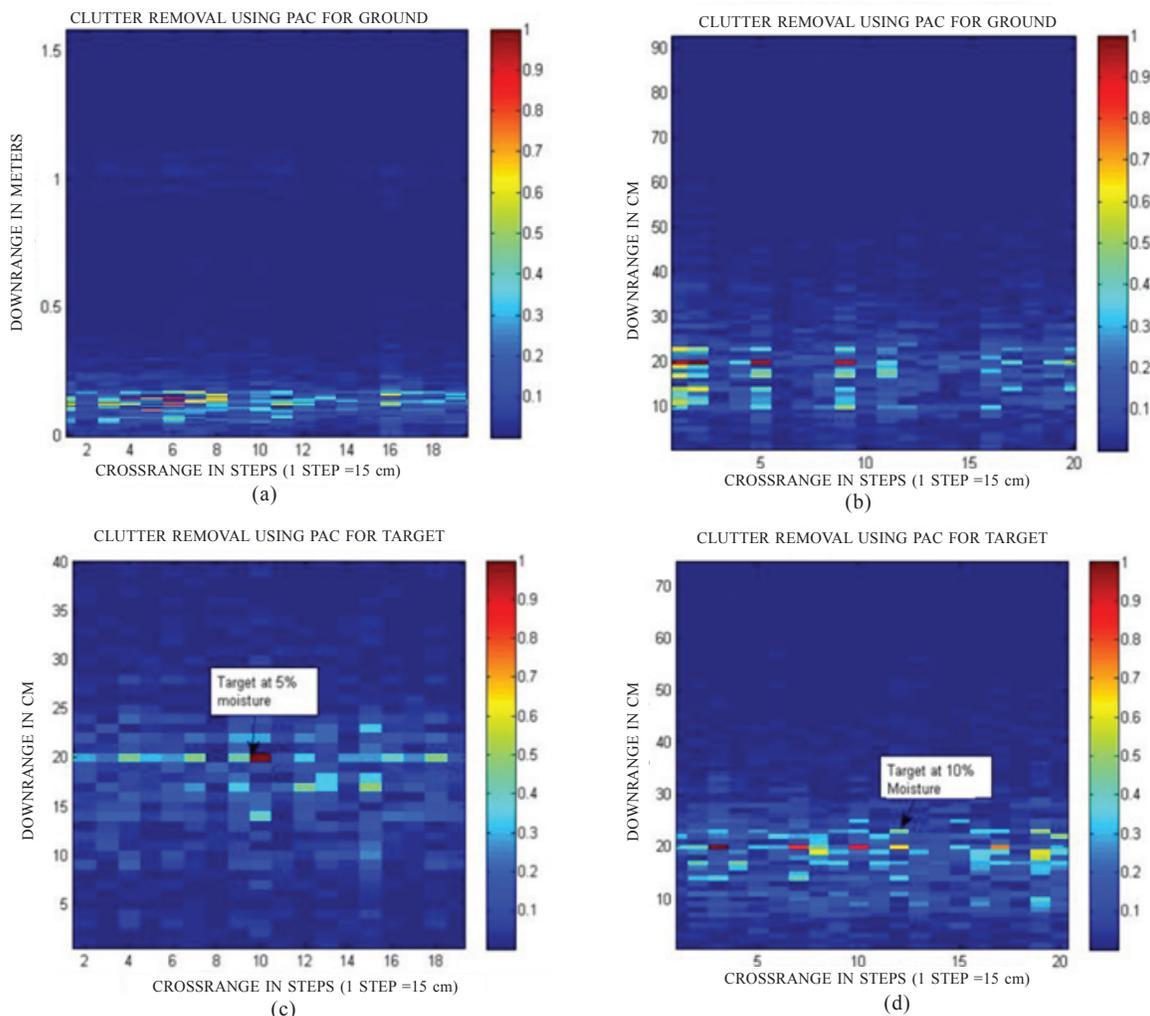
**Figure 10. PCA via SVD method: (a) without target (5% moisture), (b) without target (10% moisture), (c) with target at 35 cm (5% moisture), and (d) with target at 35 cm (10% moisture).**
