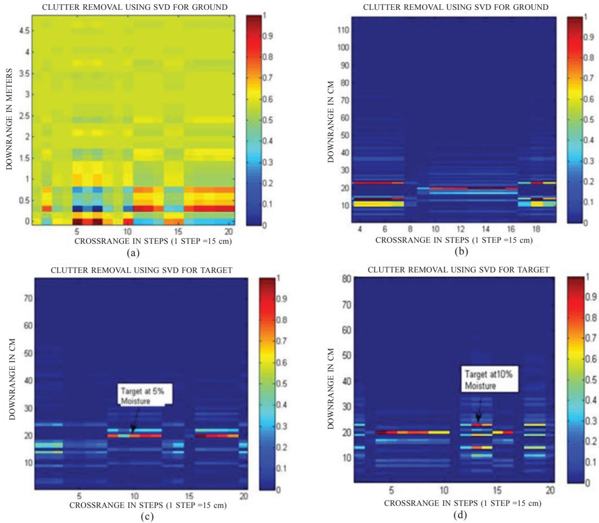
**Figure 9. SVD based background subtraction method: (a) without target (5% moisture), (b) without target (10 % moisture), (c) with target at 35 cm (5% moisture), and(d) with target at 35 cm (10% moisture).**
