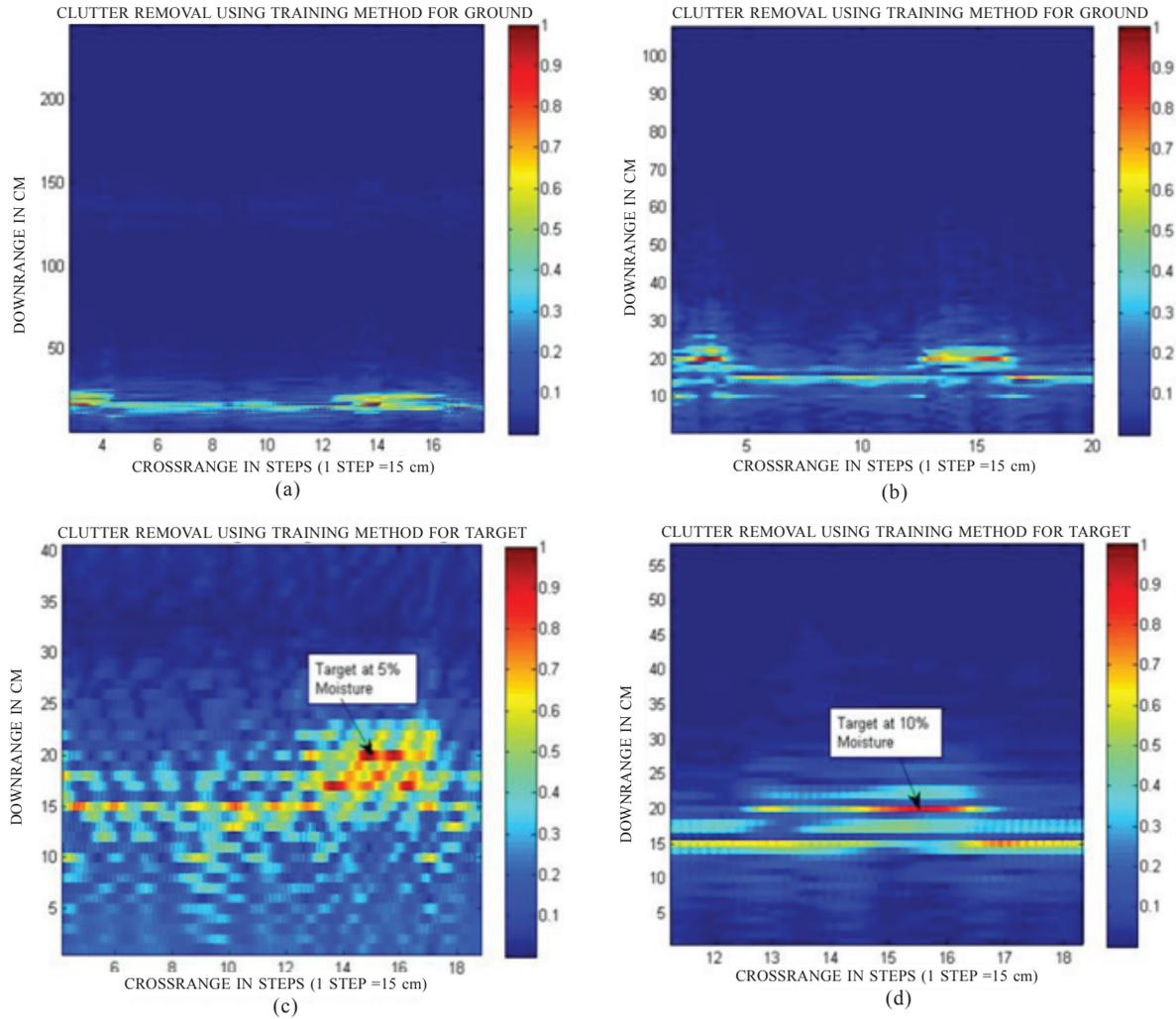
**Figure 13. Training method: (a) without target (5% moisture), (b) without target (10 % moisture), (c) with target at 35 cm (5% moisture), and (d) with target at 35 cm (10% moisture)**
