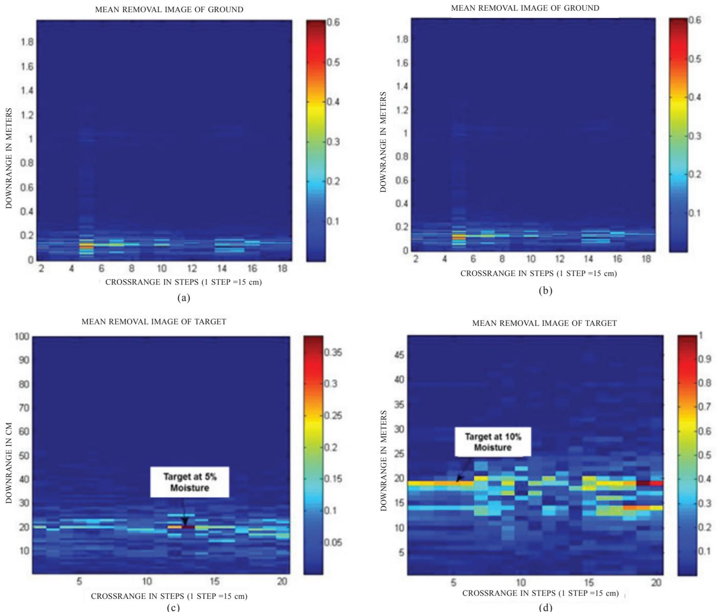
Figure 7. Mean removal method : (a) without target (5% moisture), (b) without target (10 % moisture), (c) with target at 35 cm (5% moisture), (d) with target at 35 cm (10% moisture).
