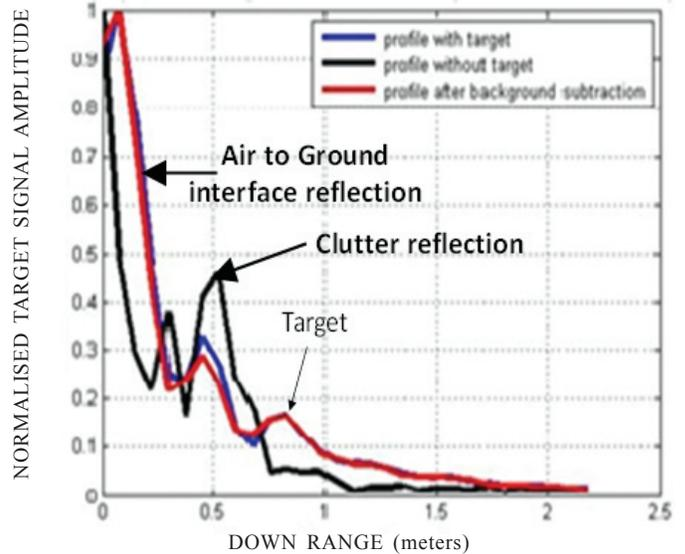
**Figure 2. A scan range profile with target, without target and after background subtraction.**
