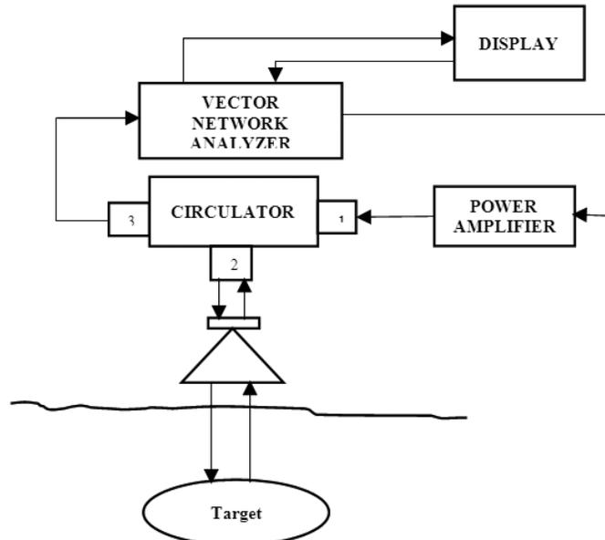
**Figure 1. Monostatic ground penetrating radar system.**
