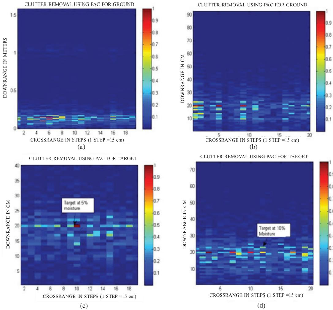
Figure 11. PCA via covariance method: (a) without target (5% moisture), (b) without target (10 % moisture), (c) with target at 35 cm (5% moisture), (d) with target at 35 cm (10% moisture).
