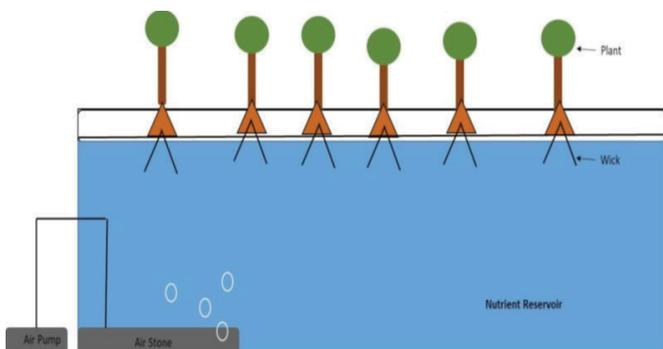
**Figure 1. Hydroponics system for plant growth. The roots are shown dipped in a nutrient solution while an air pump is used to regulate air in the nutrient solution for proper aeration of the roots. (based on information by Gonzalez, et al (2022)<sup>15</sup>).**
