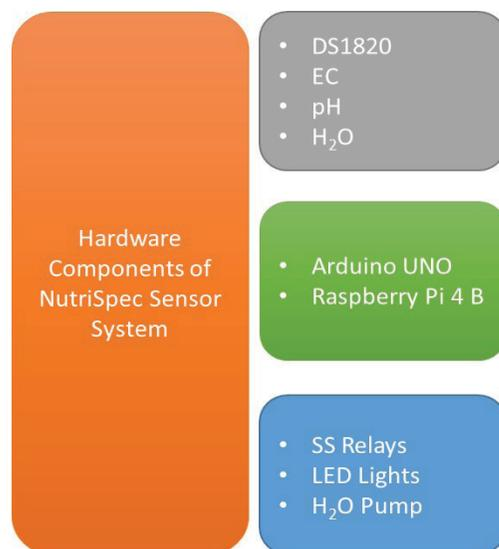
Figure 3. Hardware components of NutriSpec<sup>30</sup>
