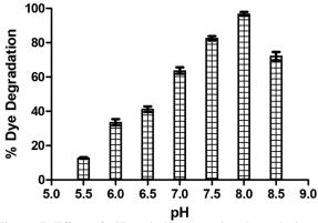
Figure 7. Effect of pH on indigo carmine degradation.
