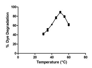
Figure 4. Impact of temperature on degradation of indigo carmine dye.
