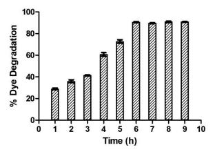
Figure 5. Impact of time on the degradation of indigo carmine dye.
