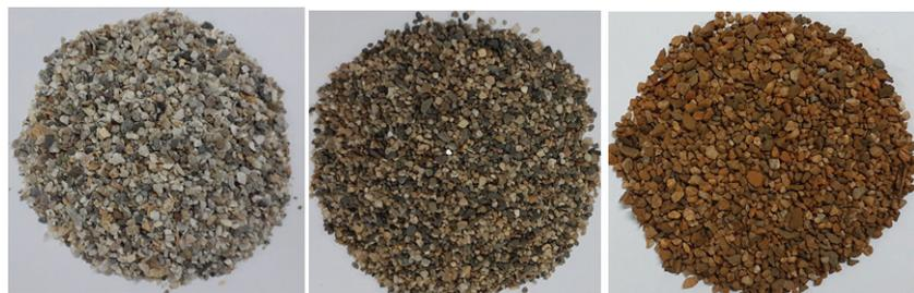
(a) Uncoated sand (b) Coated sand (c) Used coated sand
