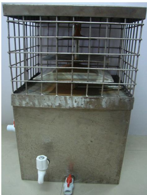
Figure 3. Non-electrical filtration system for iron removal (stainless steel).
