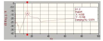
Figure 4. A typical acoustic spectrum with the help of acoustic impulse instrument.
