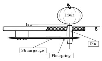
Figure 1. A typical mechanical thumb equipment.
