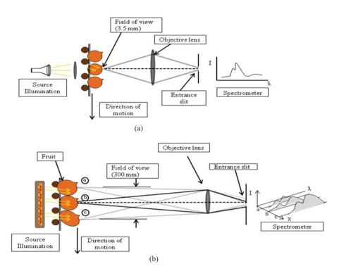
Figure 3. Sequential points in a continuous NIR system: (a)Typical mono and (b) Multiple.
