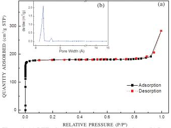
Figure 1. (a) BET adsorption and desorption isotherm (b) Pore size distribution of 13X.
