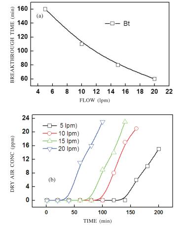
Figure 6. MeS experiment (a) Bt profile of MeS as function of flow (b) MeS concentrations in dry air.
