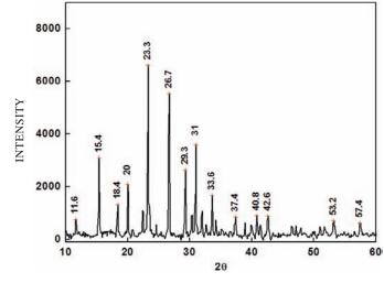
Figure 2. X-ray diffraction pattern of 13X molecular sieves.
