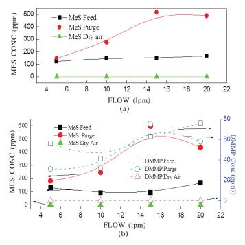
Figure 5. PSA feed, purge and dry air concentrations for 40 min (a) MeS (b) 5 per cent (v/v) DMMP in MeS.
