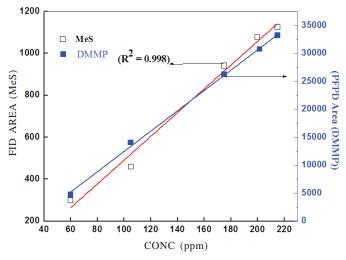
Figure 4. Calibration curves of MeS and DMMP.
