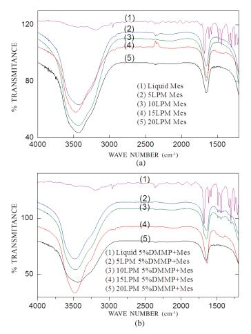
Figure 8. FT-IR of (a) MeS (b) 5 per cent (v/v) of DMMP in MeS adsorbed 13X molecular sieves.
