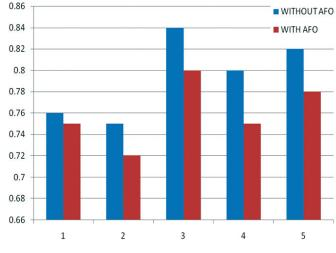
Figure 9. Stance time difference with and without AFO.
