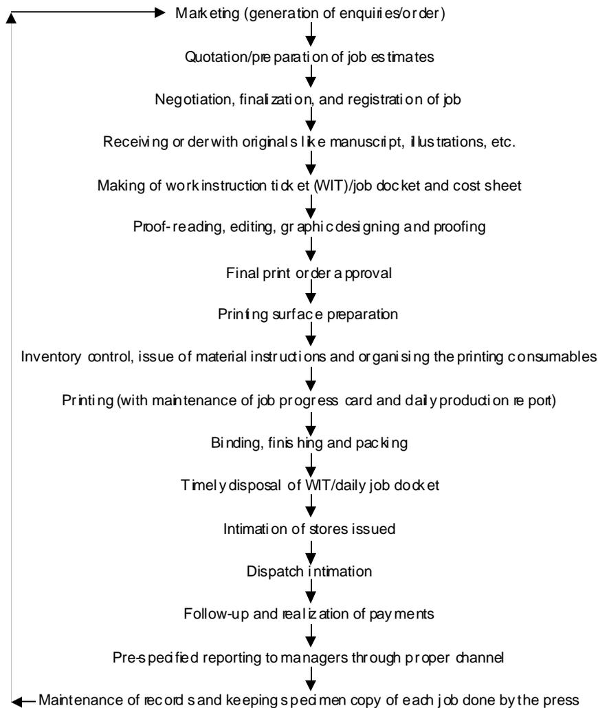
**Figure 3. Standard Press Management Routine Flow Chart**
