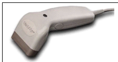
Figure 3. Hand-held barcode scanner CCD
