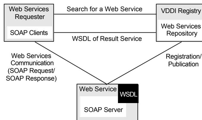
Figure 1. Basic web service architecture.<sup>4</sup>
