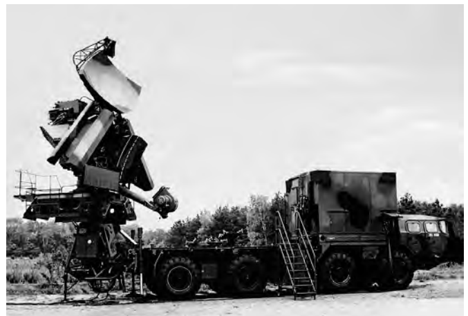
Figure 4. Rocket homing station (NEWA SC) of (SA-3) system. (WZE S.A. photo)
